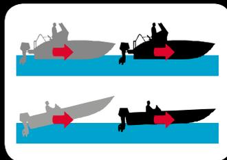
The ALUCAT does not "plow" the water but instead takes advantage of water's natural buoyancy. There is no planing threshold.
