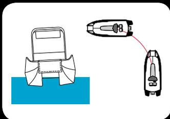
When turning, the ALUCAT stays firmly horizontal. The horizon is not lost and no blind spots are formed. Visibility remains good in every direction at all times.
