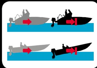
In emergency stops the ALUCAT's stern does not go down, which prevents the formation of a dangerous stern wave.
