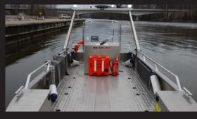
Lockable seatboxes for equipment and even deep seatboxes for divers bottles. The boats are equipped with the mounting rails and accessories desired by the customer. The self-draining deck is easy to keep clean.
