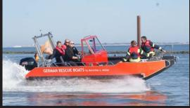
manoeuvrability and it can be driven straight ashore due to shallow draught. The diving and rescue action are possible with a wide bow ramp.
