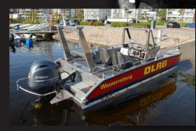
with the customer's need. Fire pump and replaceable ashore reinforcements are available. Fast to load on an ALUCAT-trailer.
